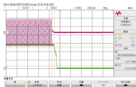
Vin=230VAC Full load shutdown (46ms)
