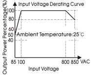
Note: 1) With an input between 85 - 100VAC/800 -850VAC, the output power must be derated as per temperature derating curves; 2) This product is suitable for applications using natural air cooling; for applications in closed environment please consult factory or one of our FAE.
